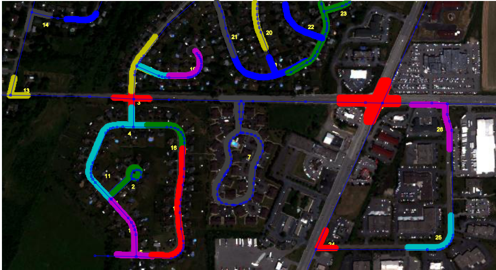
Figure 3: Sample results from the detection of intersections and curvy roads in an image using OpenStreetMap data. Different colors represent different templates that have been matched. The process has identified the major intersections in this image. Notice that the templates try to match the width of the roads as well.
