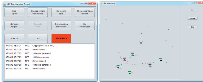
Fig. 3. Left: the console GUI. Right: The supervision window, showing current UAVs' positions
