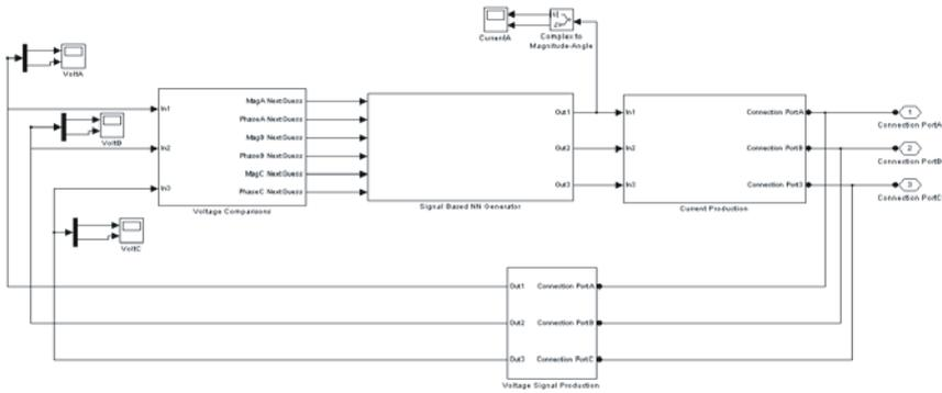
Fig. 4. Neural network test system for electrical generator
