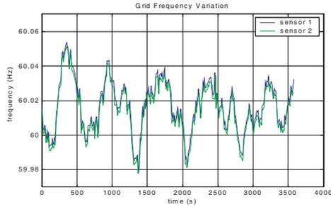
**Fig. 1.** Grid frequency variations at two locations in the power grid separated by 650 mi. NTP and post-processing techniques were used to synchronize time stamps of the data to within  $10\ \mu\text{s}$ .
