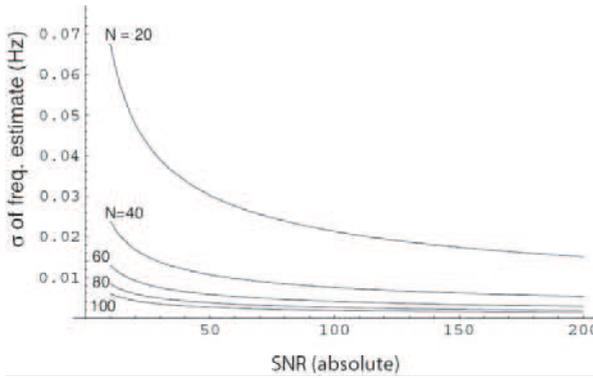
**Fig. 2.** Cramer–Rao lower bounds on the variance of the error for estimates of the signal frequency based on 1200 samples per second (20 per period) of the 60 Hz power signal with additive white Gaussian noise
