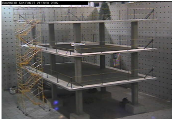
Fig. 6. Image of the test structure (30 × 50 × 35 feet) at the Bowen Lab for Structural Engineering at Purdue University. The structure will be subject to a variety of external loads and responses will be used to validate model reduction and simulation frameworks. A live web-cam image of this structure is posted at http://newton.ecn.purdue.edu/ ce/Bowen/Webcam/
